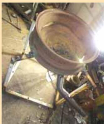
Isaac Voeller built a homemade forge out of an old wheel rim and exhaust tubing.
