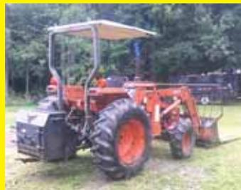
I previously sent you a picture of a heavy wood stove insert that I repurposed as a tractor counterweight by fitting it to my 3-pt. hitch. I've since welded a trailer hitch to the stove, so I have a drawbar again without removing the counterweight. I also fitted the tractor with the roof of a golf cart. **(Pete Jordahl, Oswego, N.Y.)**
