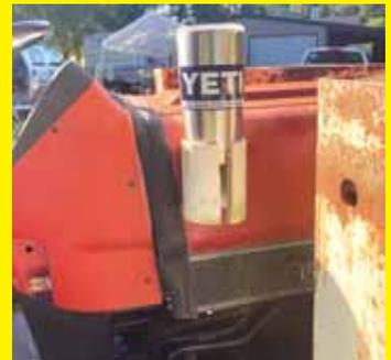
My redneck Yeti cup holder was made from a piece of pvc pipe. I just cut a slit in one side, so it expands to grip tight, and then attached it to the side of the tractor. **(Clotfelter Farms, Bogart, Ga.)**
