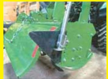
When rototilling beside small plants, dirt would spill out and bury the plants. So, I installed a shield (the black triangle in the photo) to prevent the problem. Worked great. **(Garnet Powers, Marsden, Sask.)**
