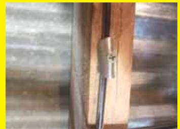
into the wood when tightened down with a wood screw. It has worked out great to hold all of my rigging gear. Should have done this a long time ago. **(Jim Williams, Leesburg, Alaska)**
