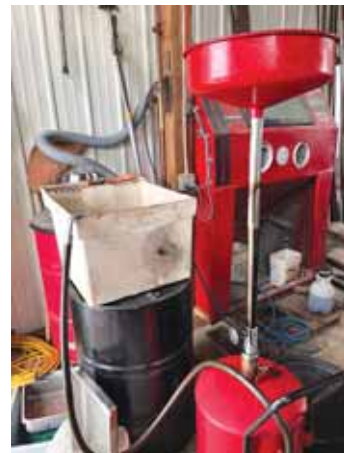
Nielsen uses an old square laundry sink as a catch basin and funnel to drain used oil into 50-gal. drums.
