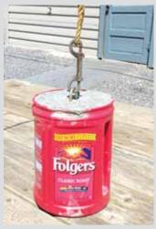
**Rick Bohl, Cedaredge, Colo.:** "I found a good use for empty coffee containers. I fill them with Sakrete and put a U-bolt in the center. Makes a great anchor for holding down canopies, tarps, or as a portable dog/ leash anchor. It's especially handy when you have to set up on a street or parking lot where you can't drive stakes."
