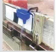
John Rochester, Deerfield, Fla.: "It's hard to hold a funnel in place when refueling my flatbed pickup. A C-clamp works great to hold the funnel steady against the sideboards. No more spills."
