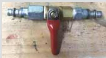
female quick coupler. Then I built an adapter using two male quick coupler fittings and a shut-off valve. Makes it quick to fill the tank by back-feeding through the hose and you can also fit the adaptor with a blow gun for cleaning off radiators, blowing out garden hoses, or cleaning an exhaust fan in your bathroom. All the parts you need can be purchased at Harbor Freight for \$12."
