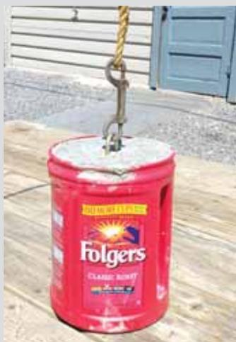
**Rick Bohl, Cedaredge, Colo.:** "I found a good use for empty coffee containers. I fill them with Sakrete and put a U-bolt in the center. Makes a great anchor for holding down canopies, tarps, or as a portable dog/leash anchor. It's especially handy when you have to set up on a street or parking lot where you can't drive stakes."
