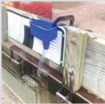
**John Rochester, Deerfield, Fla.:** "It's hard to hold a funnel in place when refueling my flatbed pickup. A C-clamp works great to hold the funnel steady against the sideboards. No more spills."
