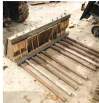
**Brue made his tractor forks using threaded pipe, angle iron, wood and u-bolts.**
