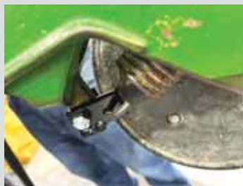
the Easy-Spring fastener, which was featured in FARM SHOW recently. It’s easy to install and repairs the worn casting hole where the closing wheel spring fastens to the corn
