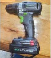
Gary Sampson, Freedom, N.Y.: "I glued a plastic piece of bit holder onto the side of my screw gun so when I have to change bits, I've got them handy right where I need them. I also glued a small bar magnet onto the battery to hold bolts and screws."
