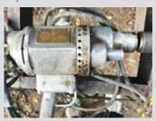
Gary Swensen, Yankton, S.D.: "My dad called this big 1/2-in. electric drill 'Big Bertha'. It's a 1938 model which was patented in 1917 by Black & Decker. It takes a big man to operate and takes two trigger pulls to start and two to stop it. If the bit gets into a tough spot, you've got to really hang on or you will go for a merrygo-round ride."
