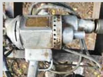
**Gary Swensen, Yankton, S.D.:** "My dad called this big 1/2-in. electric drill 'Big Bertha'. It's a 1938 model which was patented in 1917 by Black & Decker. It takes a big man to operate and takes two trigger pulls to start and two to stop it. If the bit gets into a tough spot, you've got to really hang on or you will go for a merry-go-round ride."
