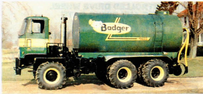
Huge spreader is equipped with 18.4 by 26 tractor tires.
