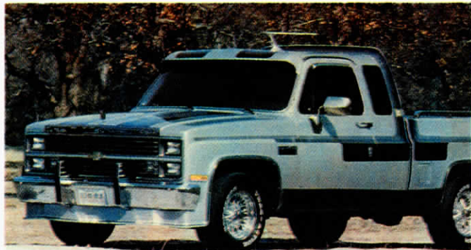
Cab is extended 16 in. to provide extra inside storage space.
