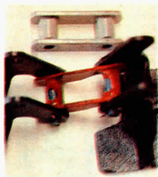
Worn connector link between paddles is replaced by new link shown at top.
