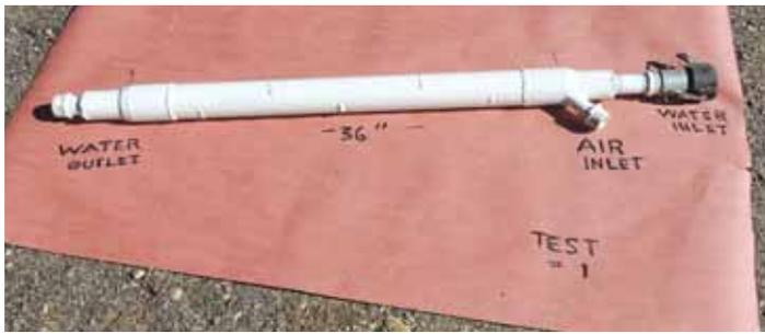
White has had the device tested by an independent lab. It tested the unit on tap water and raised DO by 137.5 percent.
