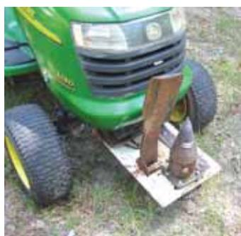
Front-mounted splitter runs off a chain drive mounted to a lawn tractor.
