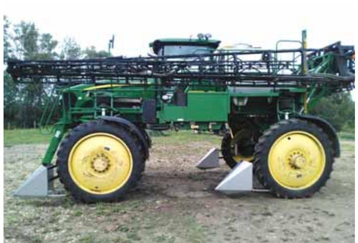
Crop protectors mount in front of lead axles and under sprayer frame and are easily raised or removed.
