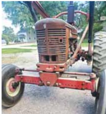
**Klahn removed the narrow front-end pedestal and fabricated a mount for the combine axle that fit in its place. He also removed the steering shaft and replaced the steering wheel on the throttle/steering wheel post with the steering wheel and motor from the 915.**
