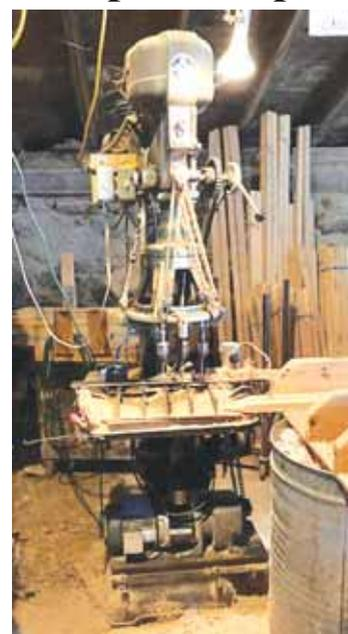
Drill press modified to drill three holes at the same time.
