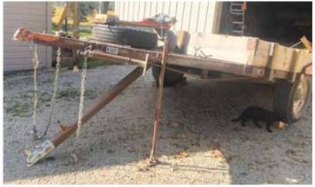
Trailer in tilt position, showing screw jack.
