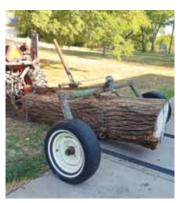
Using parts that came from equipment left on the farm, it didn't cost the amateur welder anything but his time. The log carrier works well and saves labor and time
