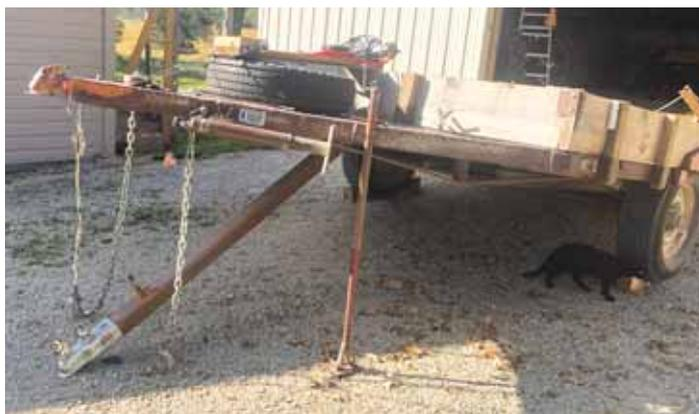
Trailer in tilt position, showing screw jack.
