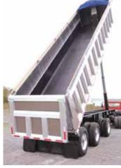
Trailer liners allow for contents to easily slide out when dumped.
