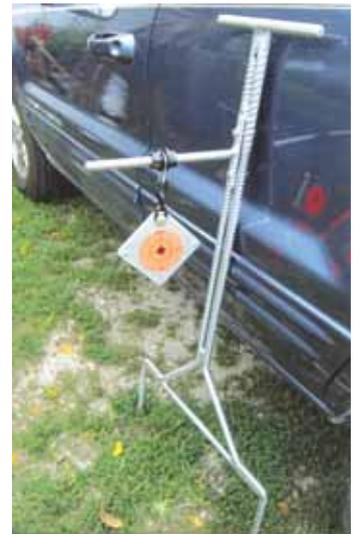
Replaceable targets are made from 4 by 4-in. metal faceplates from electrical boxes. The support post is 42 1/2 in. long with a horizontal base ending in two 8-in. pins for stability.
