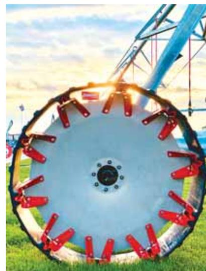
Field tests showed that wheel track depth is 30 to 50 percent less than standard 11.2 x 38-in. tires in similar conditions.
