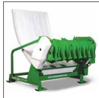
Bales sit on a lift tray that moves up and down with hydraulics. The tray moves the bale into two rotating drums with flails. The drums are a patented rotor system with 3-to-1 timing.
