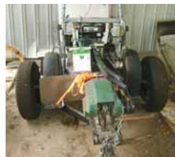
Stump grinder has a 13-hp. Harbor Freight engine and two electric motors on a 12-volt battery for driving and steering.
