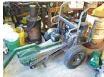
Rawls built a two-wheel trailer for his stump grinder.
