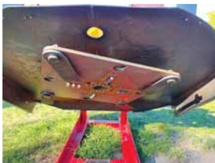
Cutting plate made of 3/4-in. thick Grade 50 steel with reinforcements on the blade mounts and center hub add strength to the skid steer-mounted Mega Mower X.
