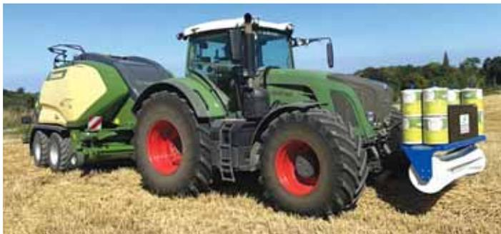
Hudson modified their existing front-mounted storage box to also be used as a swath roller and twine wrap carrier.
