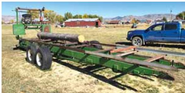
Refurbished sawmill mounted to a bale carrier frame is 25 ft. long.
