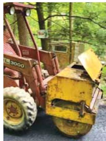
Rear roller from asphalt roller converted to skid steer quick attach.
