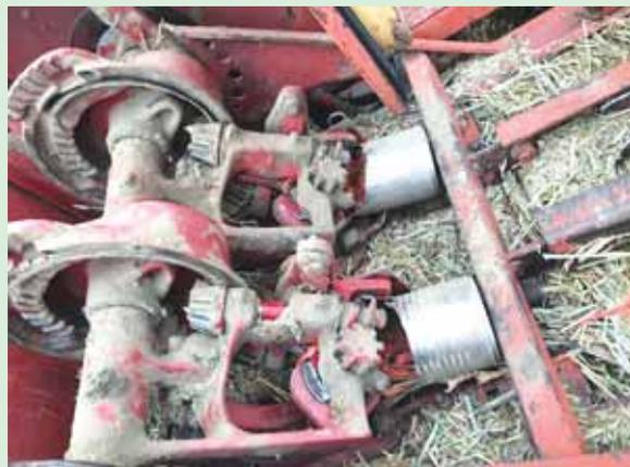
**"Cans ride on the frame behind the cutters and every time the baler makes a tie, the small cuttings fall into the cans by gravity," Arko says.**
