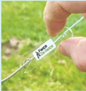
**Fence De-Fence tool allows electric fence wire to be moved for easier clearing without being shocked.**
