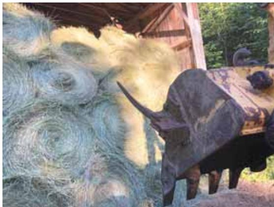
Merkley reinforced the bucket with steel plate, then attached the bale spear.
