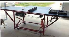
Bond's 6-ft. by 12-ft. worktable folds to 3 ft. by 6 ft. for storage and has a table saw and two routers.
