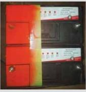
"When I get a new battery, I block off the positive post area with masking tape and then paint that area red. I believe it's a great safety measure and simple to do. I hope this idea will prevent an explosion or acid burn."
