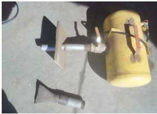
Air tank is 12 in. diameter and 24 in. long and has a 2-in. ball valve. It's used to clean air filters and set tire beads.
