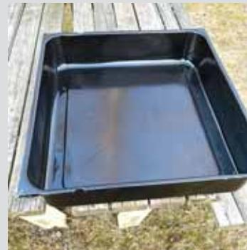
**Mark Yax, Solon, Ohio:** "I had an electric stove that I was tossing out. When removing the bottom drawer, I noticed that the stamped steel tub would make a nice drain pan or parts washing tub. I removed the front door panel and cut off the ears that held it on with my angle grinder. The only other thing I had to do was to weld up some small holes. This should work well for changing the oil in some of my equipment as it holds quite a bit. I will also use it for cleaning some larger parts."
