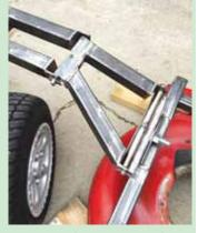
Each walk-behind mower deck got its own frame bolted to it. These frames hinge to the main frame, providing articulation up and down.
