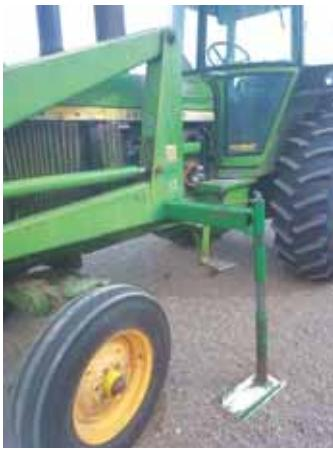
His DIY loader stand works great with his Deere 58 loader and the 4430 he mounts it to. "The key is to make the outer tube long enough to clear the front tires when you back the tractor away," says Erdman.
