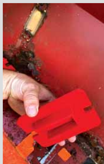
Pancoast uses a 3D printer to make seed stop covers for his drill.
