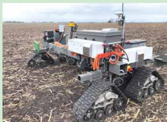
**A 5-kW electric motor powers each of four gearbox-driven track systems. Motor power is supplied by a 350-lb. 10-kW hour lithium iron phosphate battery which holds about a 90-min. charge while continuously planting.**
