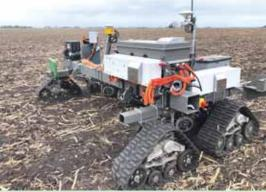
A 5-kW electric motor powers each of four gearbox-driven track systems. Motor power is supplied by a 350-lb. 10-kW hour lithium iron phosphate battery which holds about a 90-min. charge while continuously planting.
