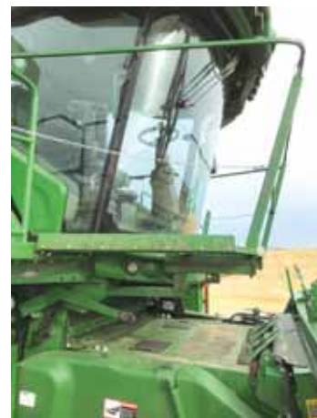
"You come out of the cab, step on the walkabout and everything's level. The top railing is 3 ft. high, and there's about 2 ft. of space in front to stand on when cleaning the windows. The railings don't interfere with viewing the swath either," says Silvernagle.
