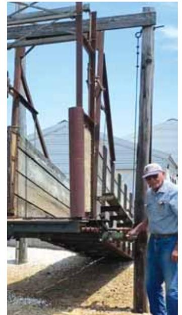
**Dennis Backhaus built an adjustable platform on the front of his loading chute that moves side to side and aligns to the door of a livestock trailer.**
