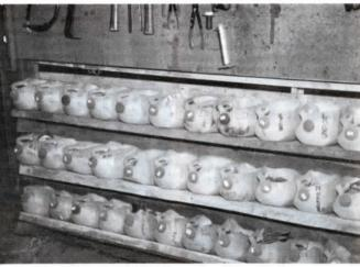
I made this handy bolt rack out of old milk jugs for holding rows of bins for bolts, nails, screws, roll pins, etc. I got the idea after putting up a peg board to hang tools and wanted to find a use for the wall space below. I made shelves out of 2 by 6's and 2 by 4's, mounting them at a slight upward
