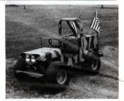
1/2 ft. long and 2 ft. wide. The rear end is off an old Sears riding mower and there's a Briggs & Stratton 3 1/2 hp. motor that mounts above it fitted with a centrifugal clutch. The body is made out of 18-ga. sheet metal. I built the frame from scratch out of 1-in. sq. tubing. My son has a ball driving it around dressed in his Desert Storm clothes. (Rick Matthews, Route 1, Box 90, Cisne, Ill. 62823 ph 618 835-2681)
