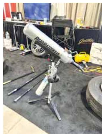
Gaither offers three models. The 3-liter BBL3L2 is designed for ATVs, motorcycles, cars and light commercial vehicles. The 6-liter BB6L2 is designed for use with motorcycles, cars, light trucks and heavy commercial vehicles. The 10-liter BB10L2 is intended for use with cars, light trucks, heavy commercial and light agricultural vehicles.
