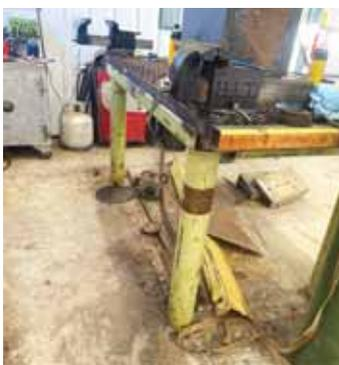
Ravenkamp used steel grate he picked up at an auction for the top, welding it to the top frame. He then welded nuts into the grate to match bolt holes in the bases of his vises.
