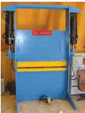
Pat Burrington's "made-it-myself" press brake produces 2,500 psi of working pressure.
