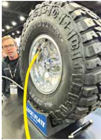
Air chuck fits standard Schrader valves. It has a rated pressure of up to 150 psi. The female end has 1/4-in. NPT threads and screws onto any standard threaded air hose.
