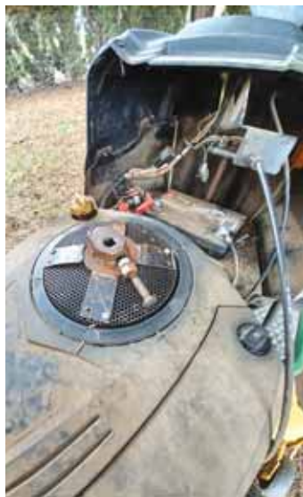
Feldman hooked an old 1/2-in. ratchet extension over the nut so he could drive it with his electric drill.
