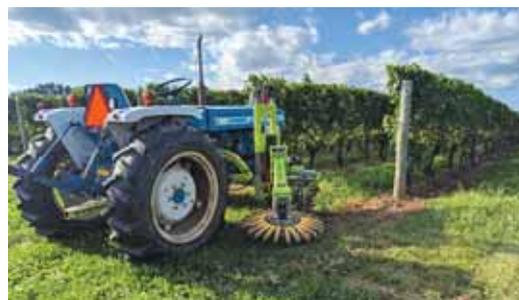
Spider discs or plates, run ahead of the 26-in. fingers and control weeds beside the trees or vines while the fingers weed within the vines. They're also mounted on a flexible arm making them safe for plants even over uneven terrain.
