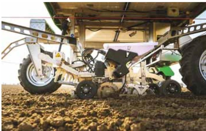
**Seeding units can do single or multiple in-line seed placements. An infrared sensor detects each seed drop and notifies the onboard computer if one is missed.**
