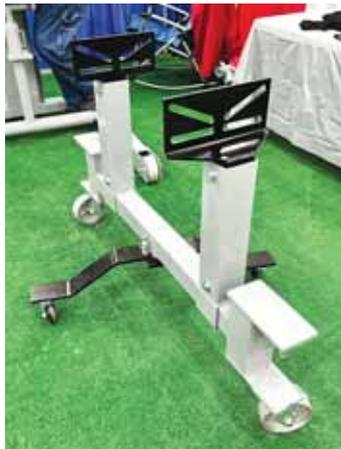
**Peters designed the splitter stand to work with tractors large and small by simply replacing the support legs. A short set works with smaller and utility tractors. A longer set fits bigger row crop tractors.**
