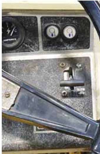
Up and down dash controls via a winch connected to the battery.
