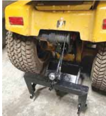
Hitch is bolted to the back of the lawn tractor transmission.
