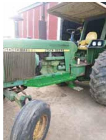
**Tractor walkway made from angle iron and safety tread plank.**
