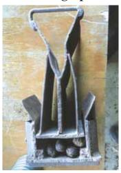
Angled wings guide the plunger, and square welds at the bottom stop the plunger from totally smashing the nuts. The 5-in. square space holds 12 or more walnuts at a time.
