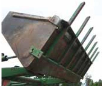
Tines are secured and welded to bottom of loader bucket.
