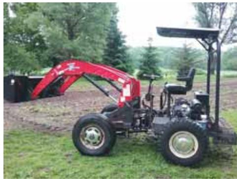
Petersen purchased a hydraulic steering mechanism designed for a Massey Ferguson tractor to control the rams on the articulation.
