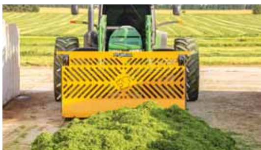
Key to the rake's design is a push plate that can be advanced forward, pushing silage or haylage off the tips of the tines.
