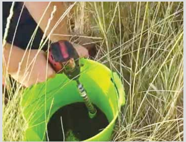
Bucket with attached pvc tube makes soil sampling easy using a handheld drill with an auger bit.
