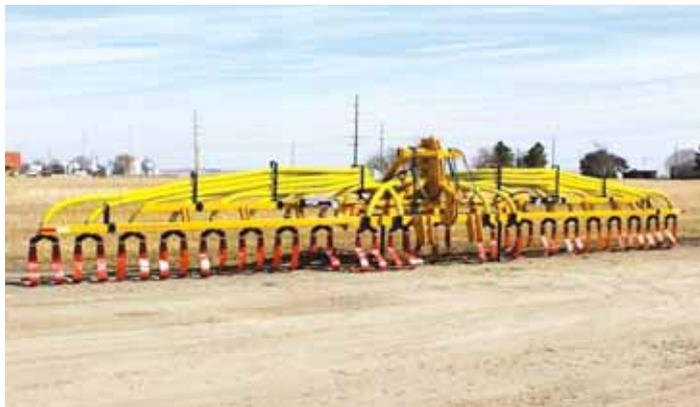
Davis says the bar's uniquely designed flux manifold features a V-shaped bottom to catch debris and rocks without plugging the product lines.
