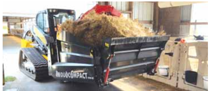
Drum processes the straw into twin blowers that shoot wheat or soybean straw, or corn stalks through the rotating pipe up to 50 ft.
