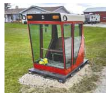
Old swather cab was attached to pallets and equipped with a small heater to make a bus stop.
