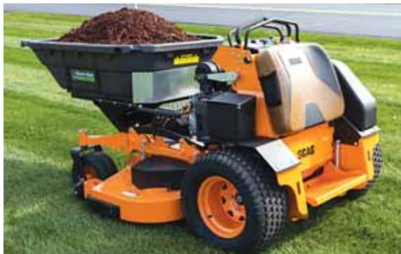
Mower Mule poly tub add-on holds 12.5 cu. ft. and can be quickly attached or removed from mower.
